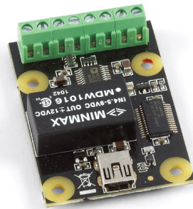
Phidget Analog Board controlled by using phidget_analog()
