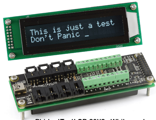
PhidgetTextLCD 20X2 : White and Integrated PhidgetInterfaceKit 8/8/8 controlled by using PhidgetTextLCD() and phidget_interface888()
